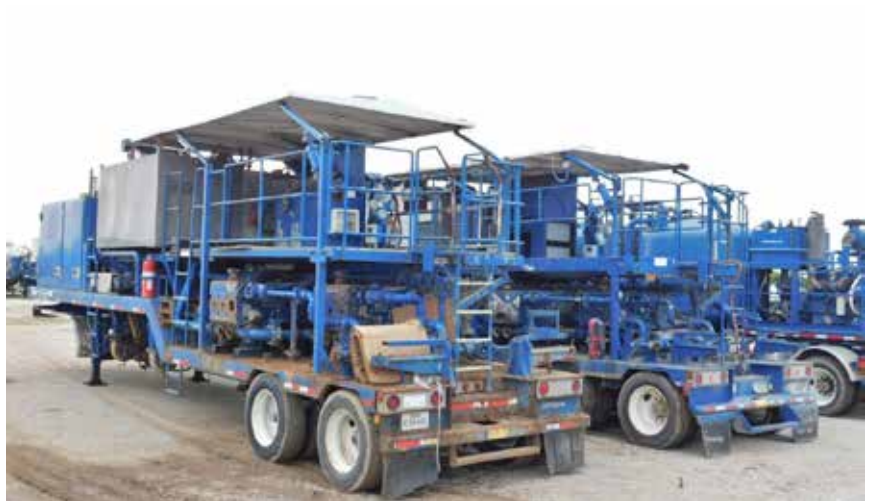
22 – Twin Cement Pumpers
